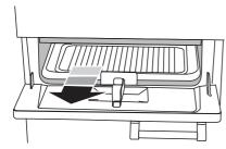
Remove the pan from the bottom of the grill compartment.
